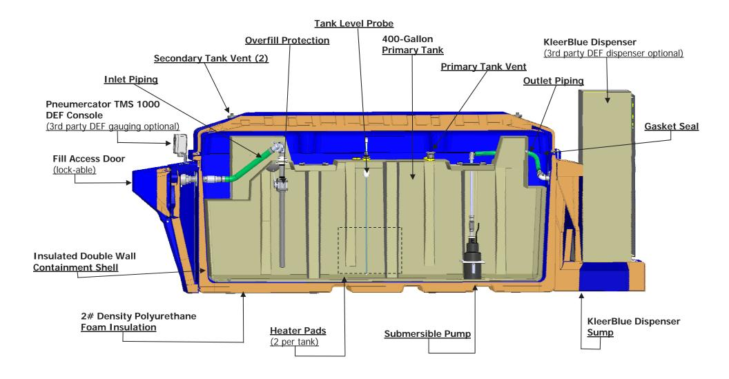
KleerBlue<sup>™</sup> 400-Gallon DEF Insulated, Heated Storage Tank, Section View Separation By Design
